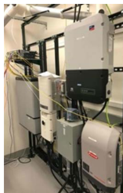
Figure 4. Inverters under test in the ARPA-E NODES experiment.
