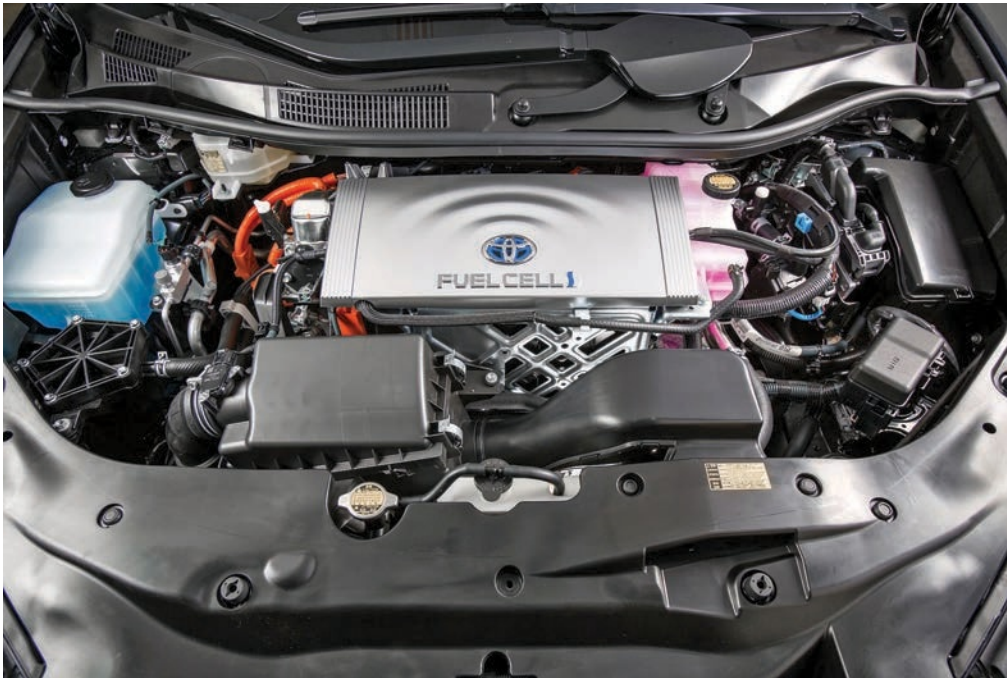
Most of the fuel-cell system components are placed low in the frame to improve the Mirai's handling.
