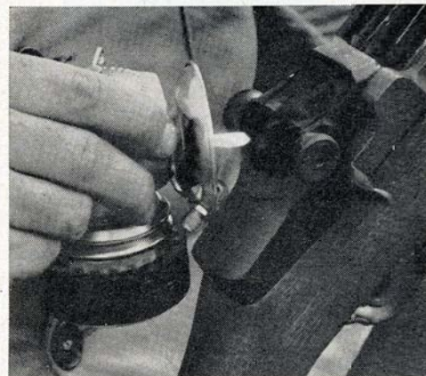
Blackening the sights with a carbide lamp will kill any glare
