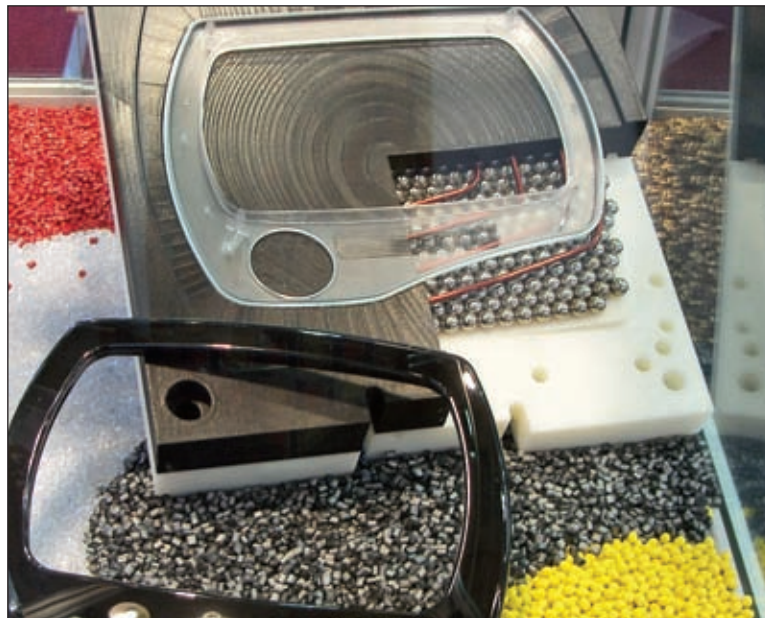
KIMW's display of a cut-away view of its close-contour BFormold ball-filled mold that shows the balls under the mold insert surface. This piece is displayed with a black high glass navigation equipment frame.
